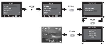
Use the  $\blacktriangleleft$  or  $\triangleright$  button to select a field, such as year, month, day, hour, minute. Use the  $\blacktriangle$  or  $\checkmark$  button to adjust the value in the field. Press the OK button after all fields are set.
